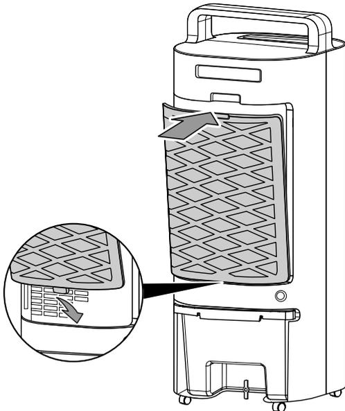
1. Remove the air filter from the device.
