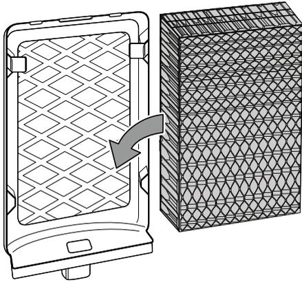
6. Reinsert the air filter into the device.
