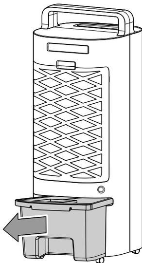
3. Fill the water tank with fresh drinking water only. Optionally, you can add ice cubes made of drinking water for additional cooling.
