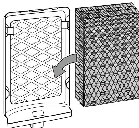
5. Reinsert the air filter into the device.
