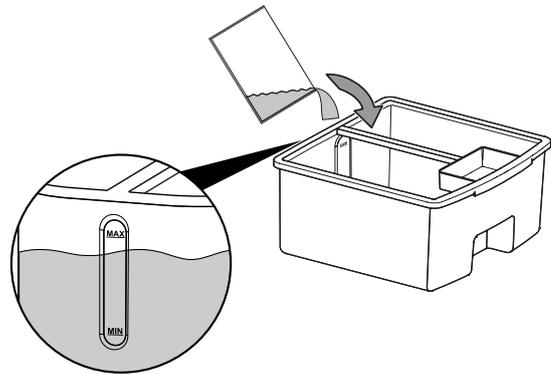
4. If required, put the ice packs into the water tank for additional cooling.
