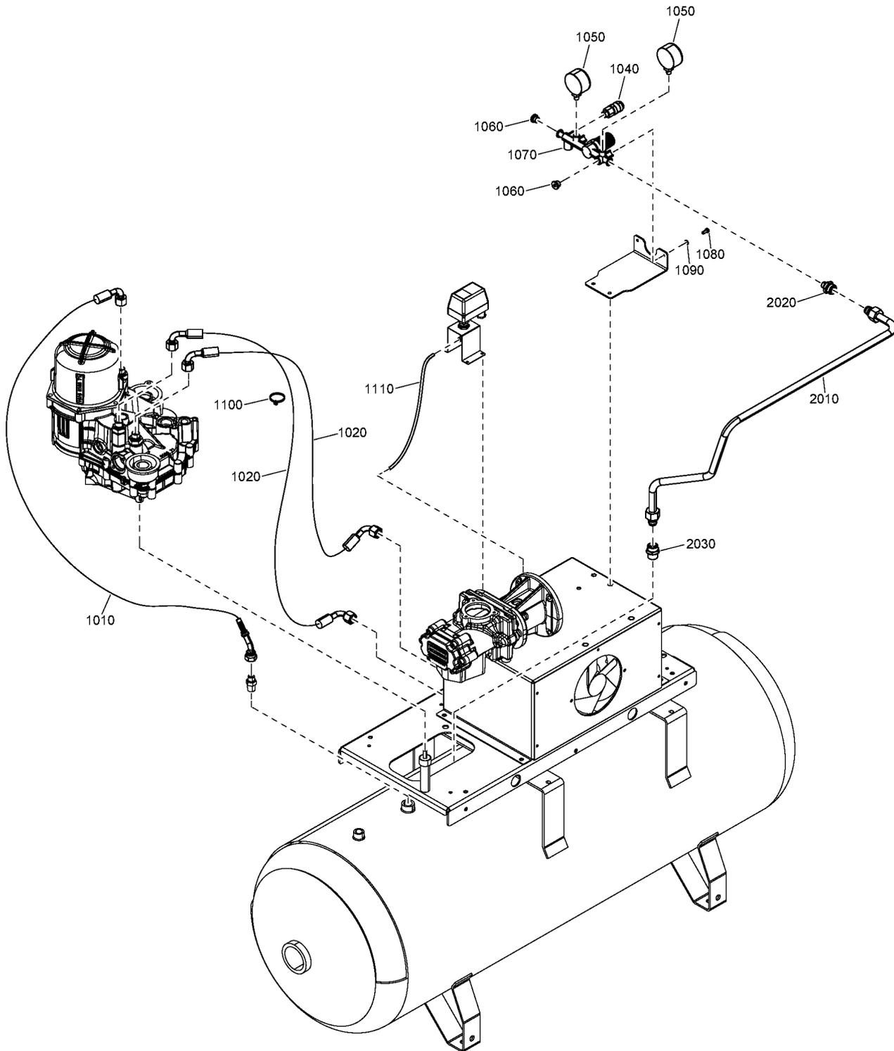
**10 - Air outlet - Tank-mounted - Air receiver 200L**
