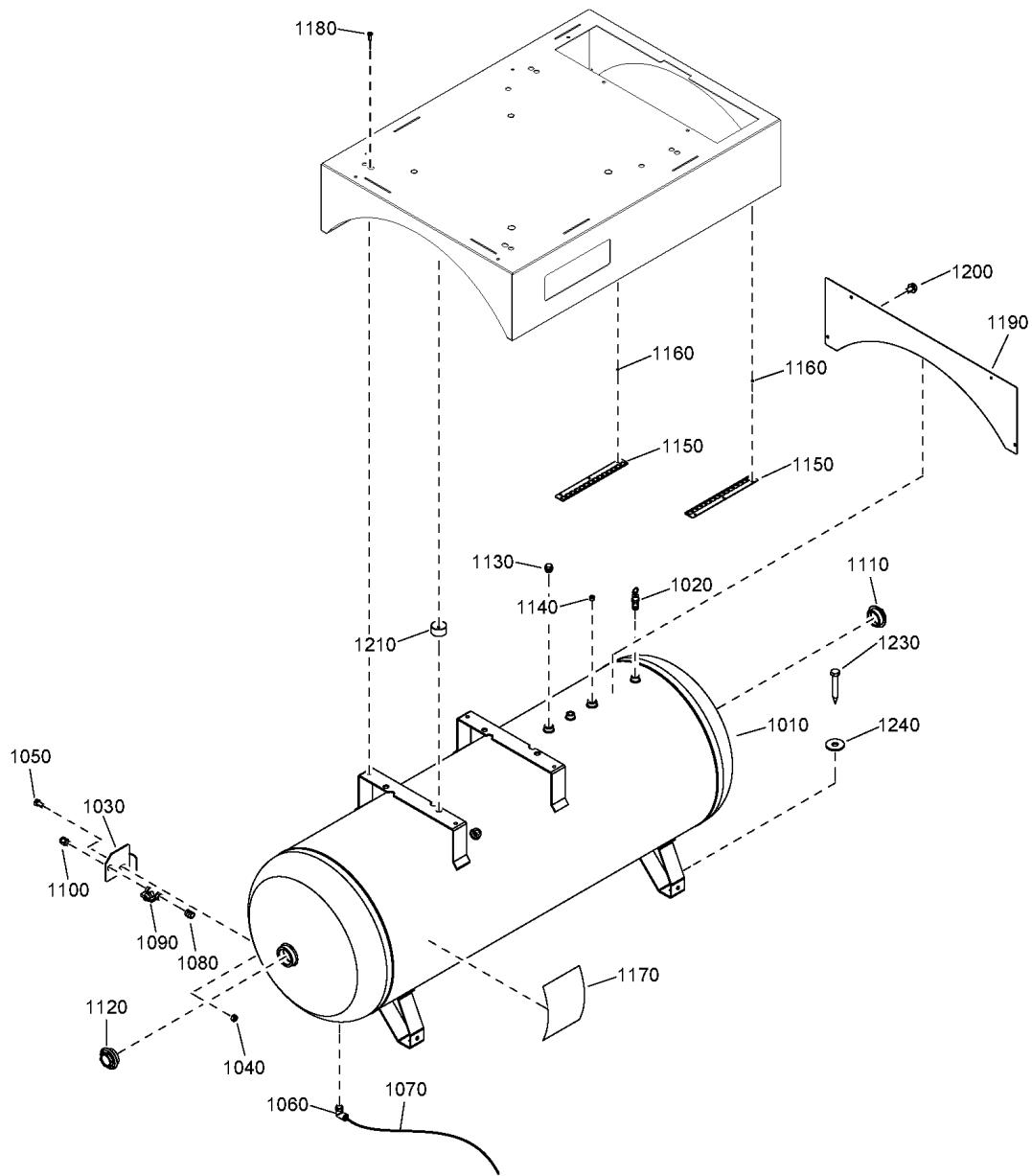
**20 - Air vessel (NS 7.5, NS 10) - (ASME, CRNASME) - Air receiver - 500L - Without dryer**
