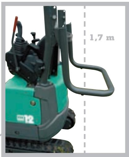
The 12VXE can drive through doors no more than 90 cm wide. The rollbar can also be removed in just a few minutes to facilitate passing through low clearance areas.
