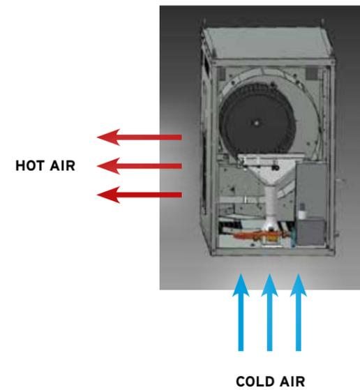
CF 75 SPARK takes air from the bottom, which is heated through a gas burner and comes out through a centrifugal fan
